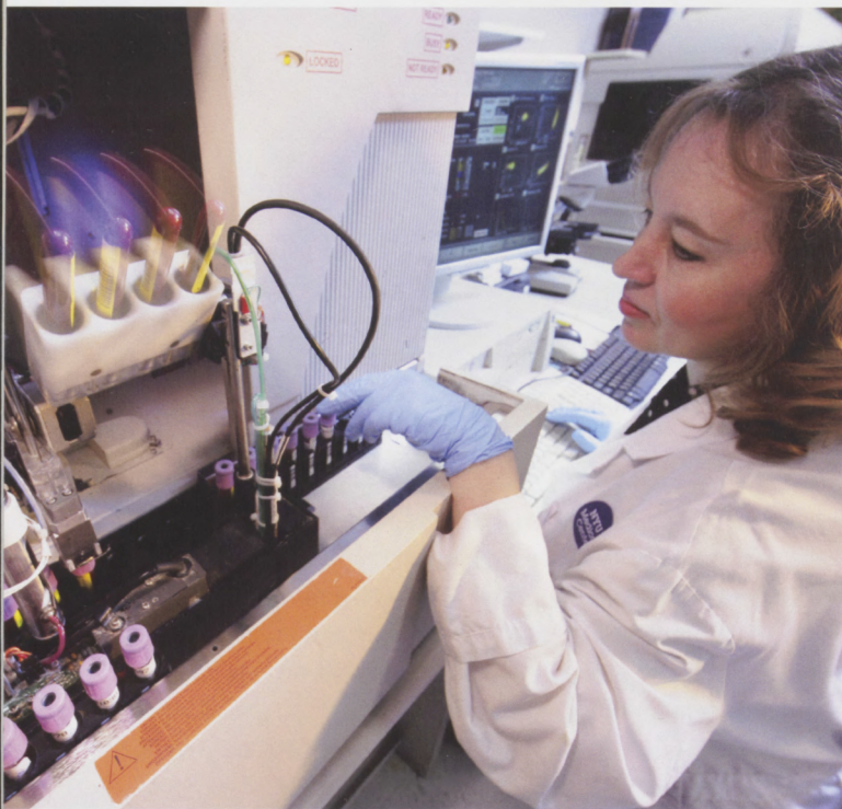
Using an automated hematology analyzer, Danuta Dembek, a medical technologist, can determine the cellular components of blood, counting thousands of cells very precisely within about three minutes.
